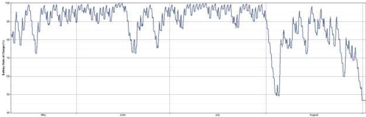
fig 19: Battery bank - 5kWh Nuuk
